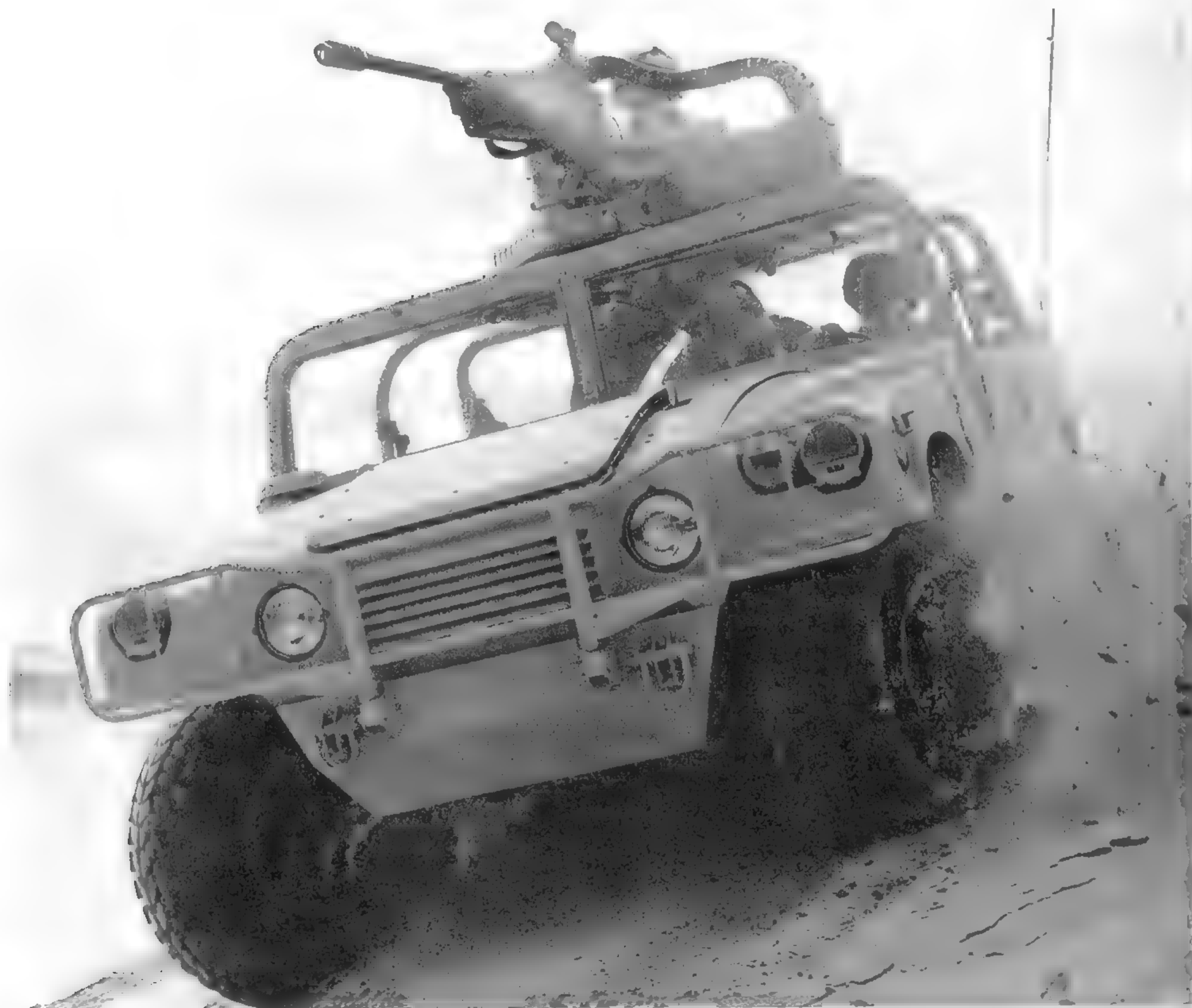
Special Operations units are outfitted with these heavily modified HMMWVs. Among the modifications was considerably increased protection for the engine compartment. Also, these are unique among U.S. HMMWVs in that they carry spare tires. Any other vehicles with spares are foreign sales units. (Photo courtesy of AM General Corp.)
